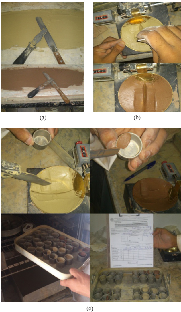
Fig. 2 Determination of the LL after 1 and 30 days of curing; (a) the paste was remixed with each stabilizer for at least 15 min before performing the first test, (b) practice the groove and start the test and (c) determination of the water content (LL) by desiccation at 105 °C during 1 day
